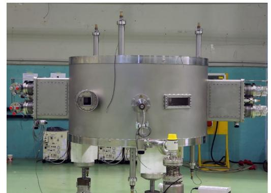
**Assembly of the magnet inside the yoke**
